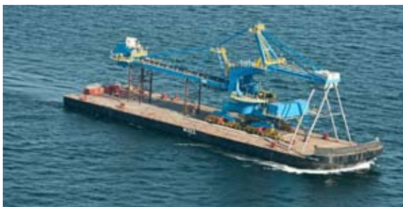
Another fully assembled EMS-Tech Stacker-Reclaimer, delivered in 2013, served as inspiration for the move on the West coast of Canada... EMS-Tech looks forward to the next big move!
